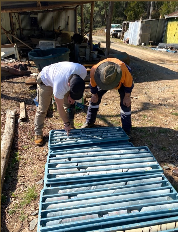
Stewart Govett and Geologist Denis Walsh inspecting some of the 223 metres of DDH core from two drill holes showing massive sulphides that may contain gold and a large quartz vein intersected with pyrites and arsenopyrites.
