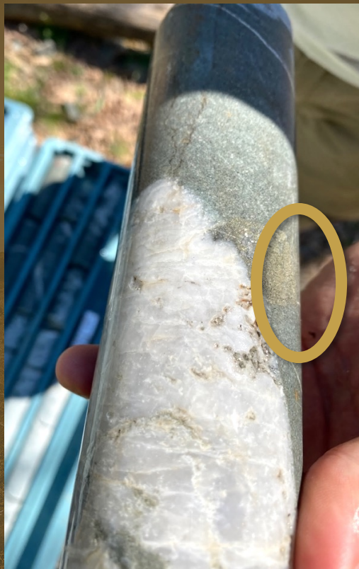
Stewart Govett and Geologist Denis Walsh inspecting some of the 223 metres of DDH core from two drill holes showing massive sulphides that may contain gold and a large quartz vein intersected with pyrites and arsenopyrites.
