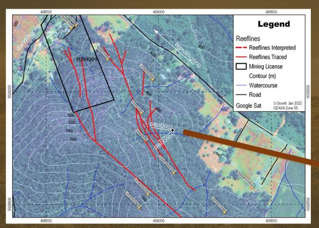
Drill holes GBDD001 and GBDD002 were drilled to test the down plunge intersections of Shaws-Home Reef and Red Leader-Home Reef. Logging and assaying of these holes are to be finalized in the first quarter of 2022.
