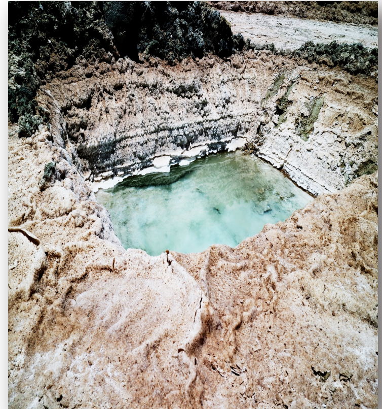
Brine pond contains 900ppm lithium in the Sodium and potassium saturated brine
